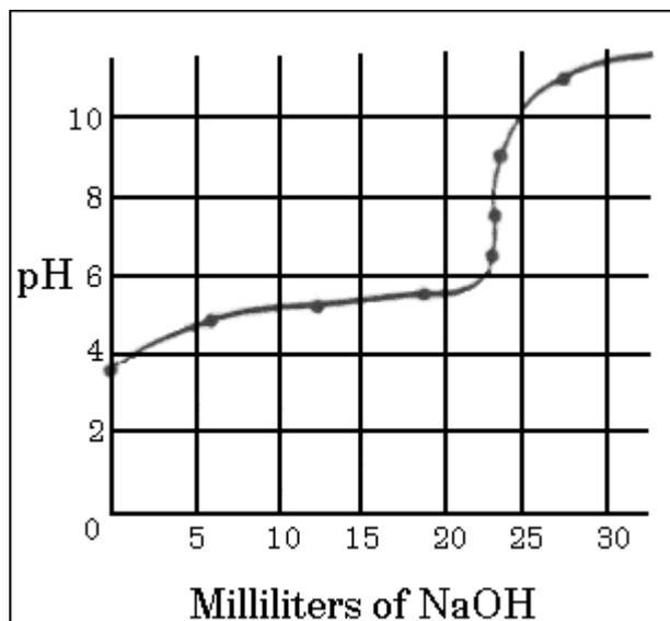
A 30.00 milliliter sample of a weak monoprotic acid was titrated with a standardized solution of NaOH. A pH meter was used to measure the pH after each increment of NaOH was added, and the curve above was constructed.
